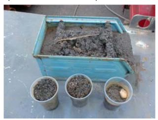
Clinker and metal remains taken out by RHC SA's mechanical cleaning tools.
