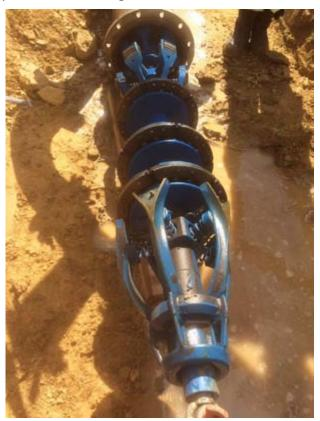
Pulling out a 12" mechanical cleaning tool
