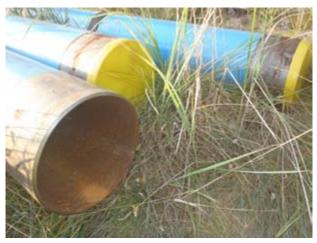
Bad storage of pipelines leading to corrosion and rust
